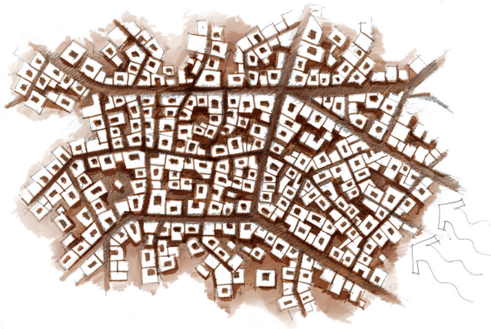
Neighborhood clusters are accessible by main spine and individual residential units are accessed through network of semi-private streets and cul-de-sacs
